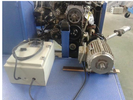
Figure 1: Motor setup, electric motor and inverter
